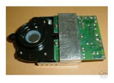
Figure 19: Ultrasonic Transducer
