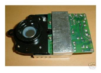
Figure 7: Ultrasonic Transducer
