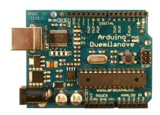
Figure 20: Arduino Microprocessor
