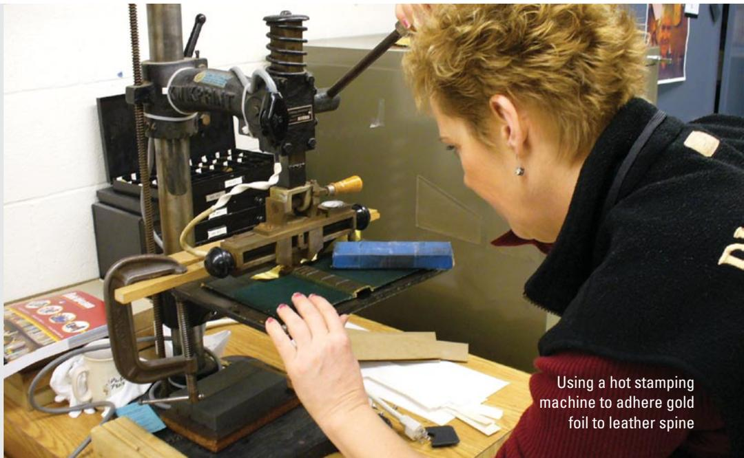
Using a hot stamping machine to adhere gold foil to leather spine
