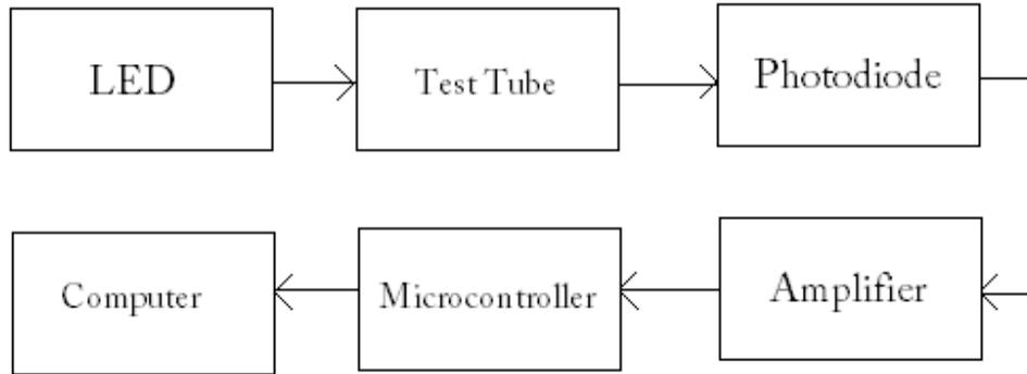
**Figure 4.3.1** Functional Design using Test Tubes
