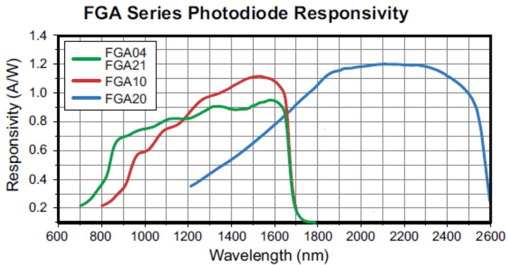
**Figure 3.5.3** Photodiode Responsivity
