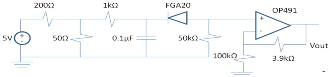
**Figure 3.7.1** Refined Photodiode and Amplifier Circuit
