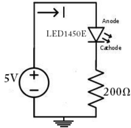
**Figure 3.5.1** Circuit for Biasing LED1450E
