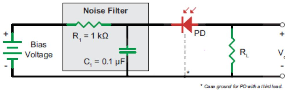
**Figure 3.5.4** Recommended Circuit Diagram
