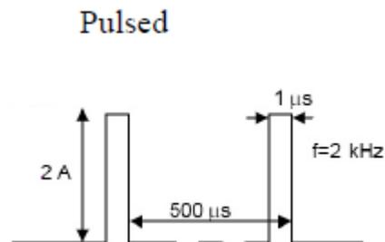
**Figure 4.4.2** Pulsed Current Used for LED2050P Operation Resulting in 28mW Power.
