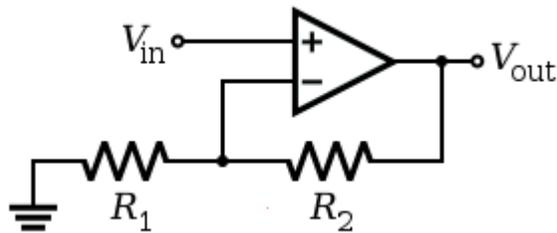
**Figure 3.5.6** Non-Inverting Amplifier
