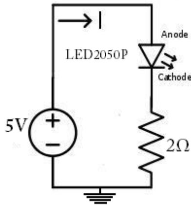
**Figure 4.4.3** LED2050P Circuit Design Resulting in  $I=2A$
