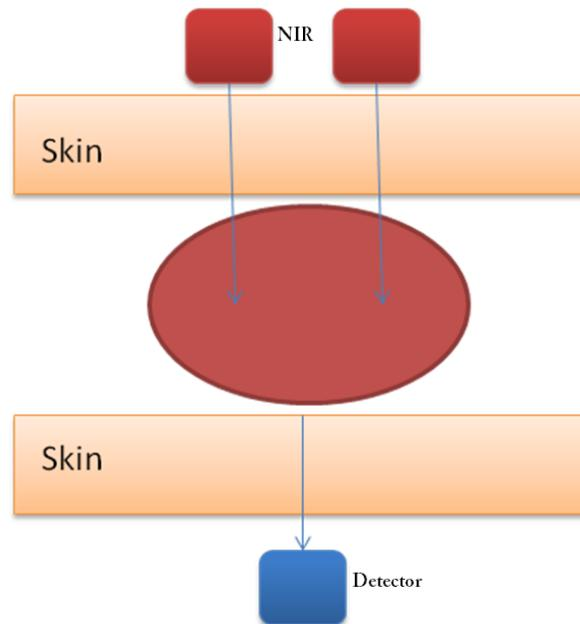
**Figure 1.3.1** Schematic Overview of Operation of Non-Invasive Blood Glucose Monitor. NIR are Near-Infrared Emitting Light Sources, Detector detects the amount of light.
