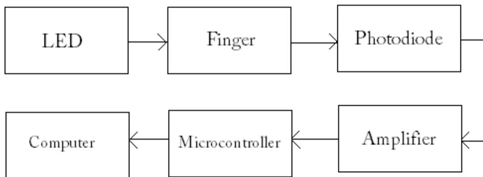
**Figure 4.2.1** Initial Projected Functional Design
