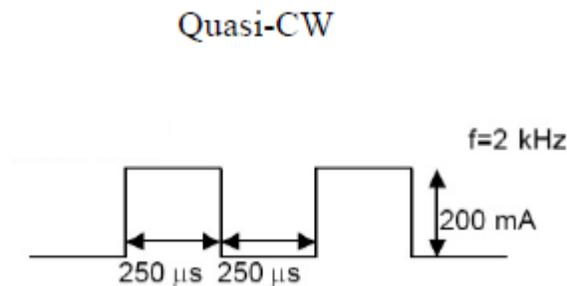
**Figure 4.4.1** 50% Duty Cycle Current Used for LED2050P Operation Resulting in 1.1mW Power.
