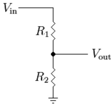
**Figure 3.5.5** Voltage Divider Circuit
