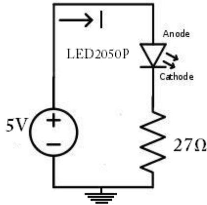
**Figure 3.5.2** Circuit for Biasing LED2050P
