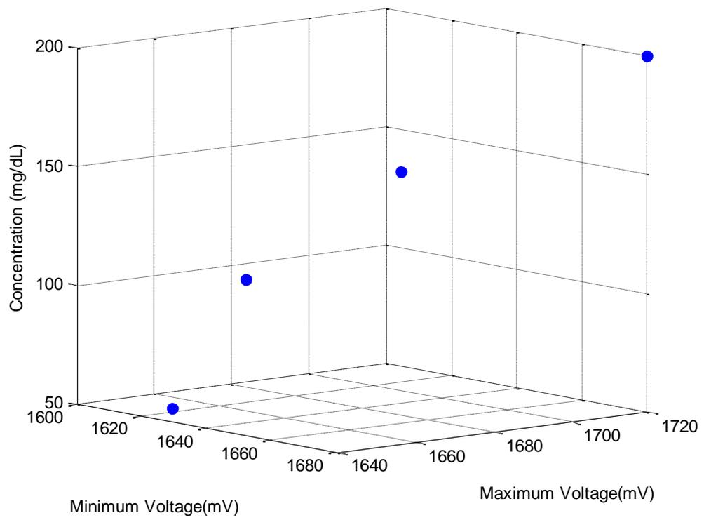
**Figure 4.5.1** Glucose Concentration versus Minimum and Maximum Voltages
