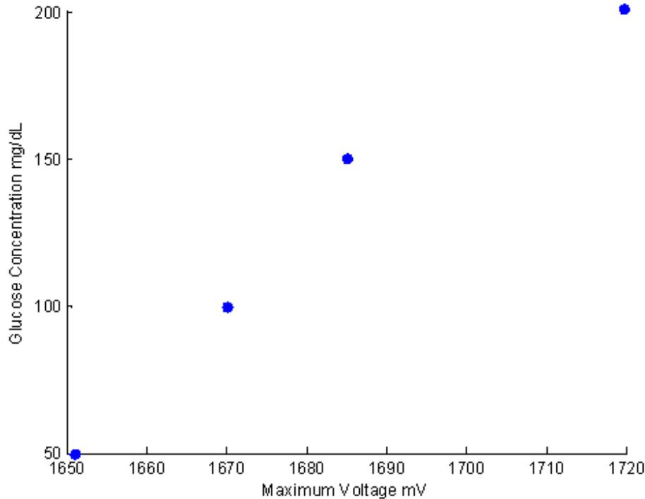
**Figure 4.3.3** Glucose Concentration versus Maximum Voltage from Photodiode
