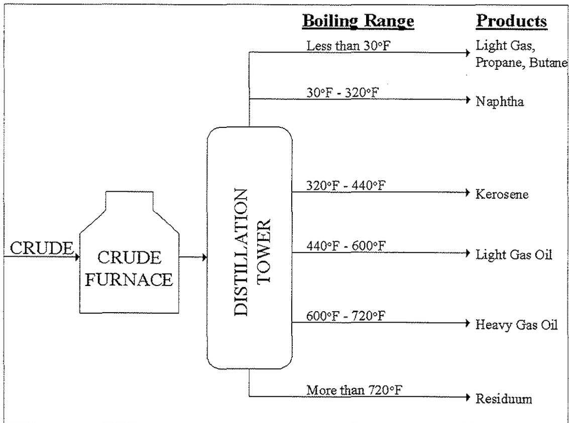
**Figure 4: Crude Oil Distillation**
