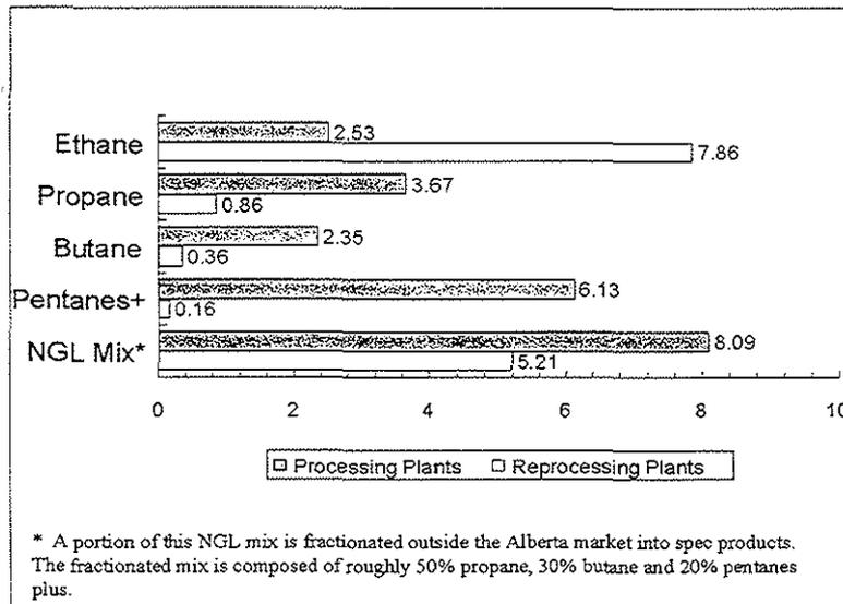
**Figure 3: Average Extraction of NGL to Inlet Gas Ratio at Processing and Reprocessing Plants in Alberta**
