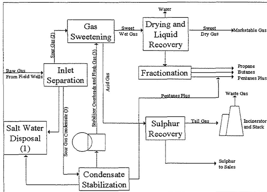
**Figure 2: Simplified Flow Diagram of a Gas Processing Plant**
