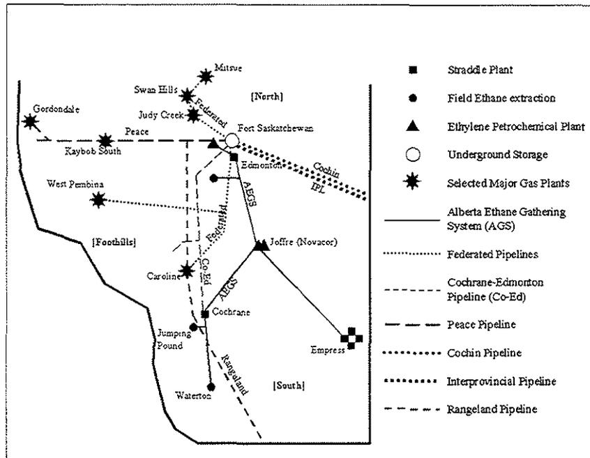
Figure 12: Alberta NGL Feeder Pipelines
