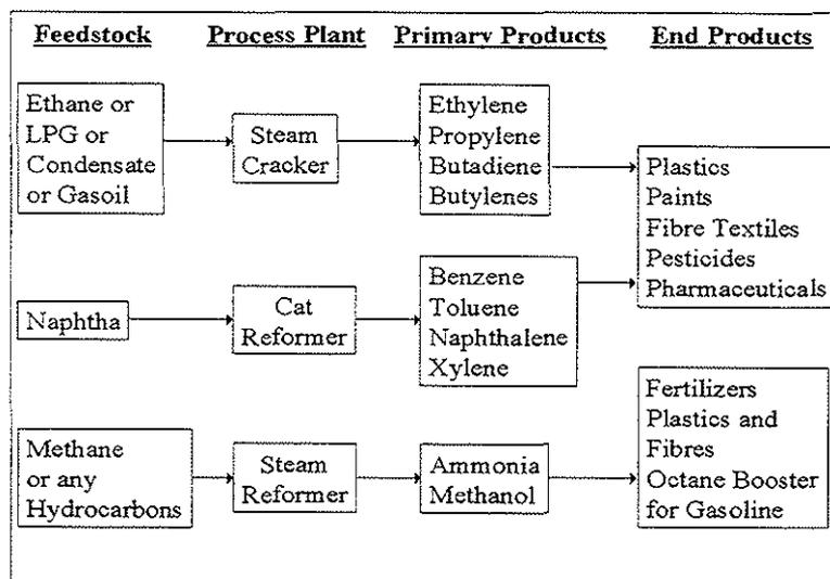
**Figure 7: A Simplified Flowchart of the Petrochemical Industry**
