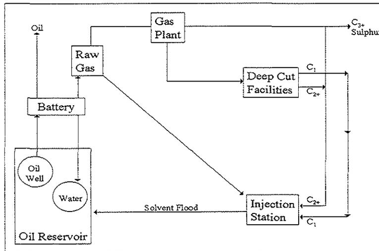
**Figure 11: Typical Hydrocarbon Miscible Flood Facilities**
