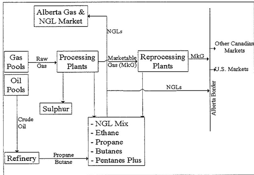
Figure 1: Simplified Schematic of Alberta Natural Gas and NGL Flows.
