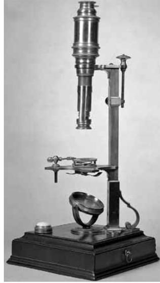
Figure 2. Microscope designed and introduced by John Cuff in 1744. Used by permission from the Wellcome Library, London.
