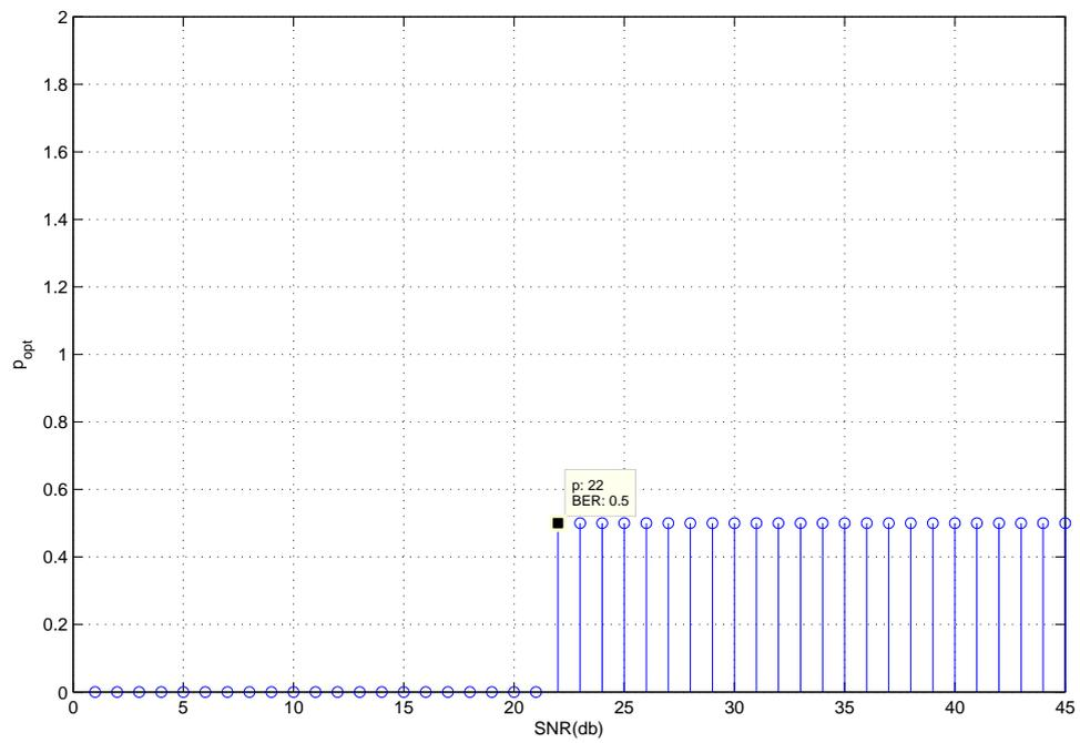
Figure 6.11:  $p_{opt}$ -SNR plot in highly correlated channels case ( $|\sigma| = 0.8$ )
