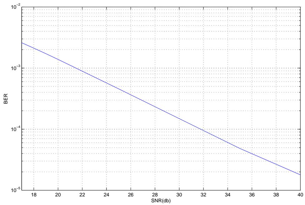
Figure 6.6: BER-SNR plot in moderately correlated channels case ( $|\sigma| = 0.2$ )
