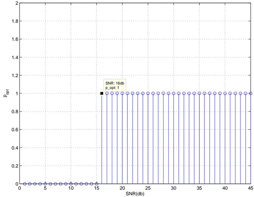
Figure 6.2:  $p_{\text{opt}}$ -SNR plot in uncorrelated channels case ( $\sigma = 0$ )
