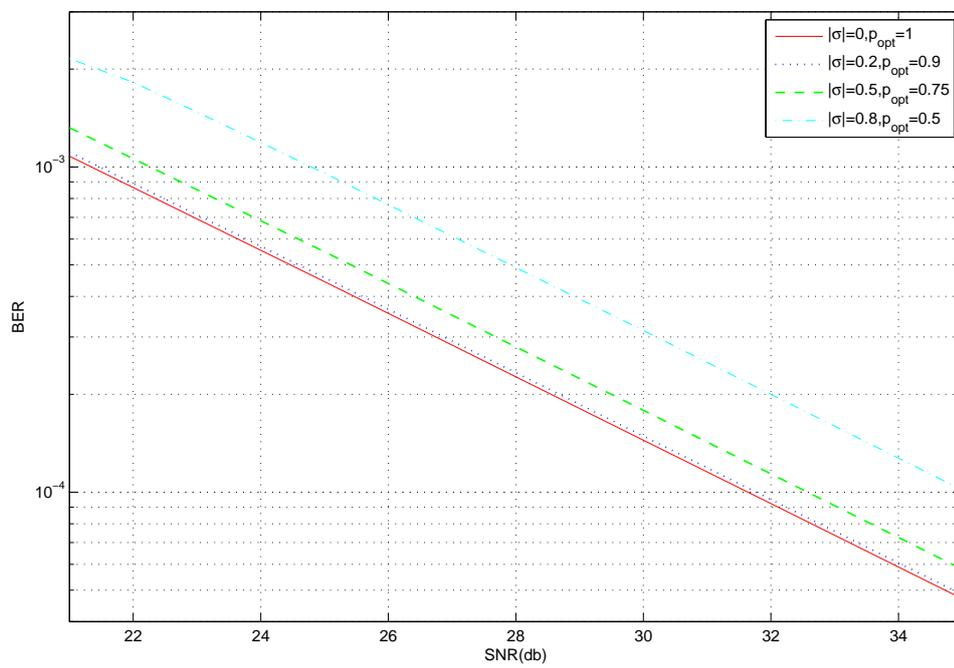
Figure 6.13: BER-SNR plot in different channel cases
