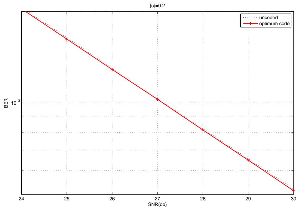
Figure 7.3: Comparison of SNR-BER when  $\sigma = 0.2e^{0.5j}$
