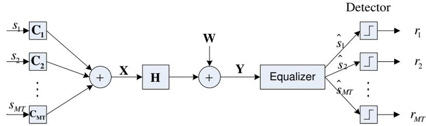
Figure 2.1: MIMO communication system model
