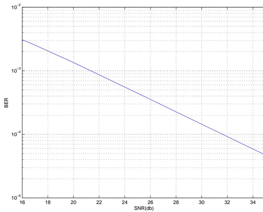
Figure 6.3: BER-SNR plot in uncorrelated channels case ( $\sigma = 0$ )
