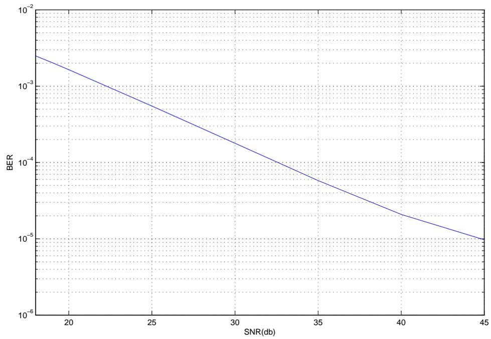
Figure 6.9: BER-SNR plot in moderately correlated channels case ( $|\sigma| = 0.5$ )
