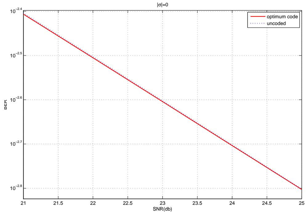
Figure 7.2: Comparison of SNR-BER when  $\sigma = 0$
