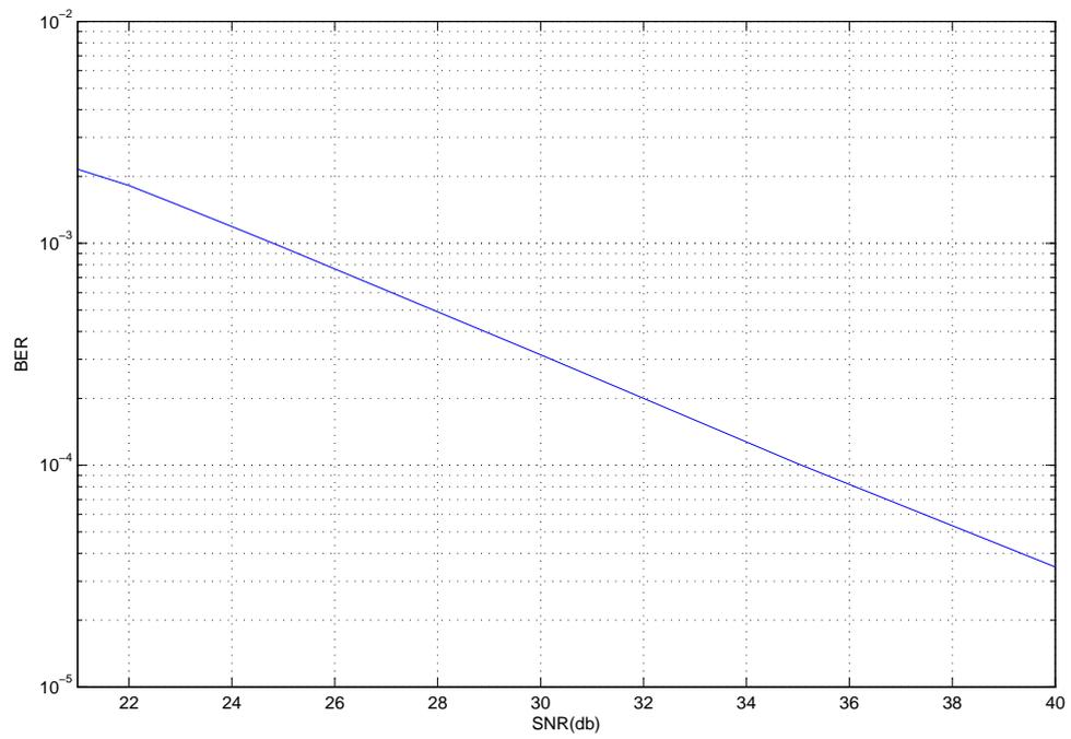
Figure 6.12: BER-SNR plot in highly correlated channels case ( $|\sigma| = 0.8$ )
