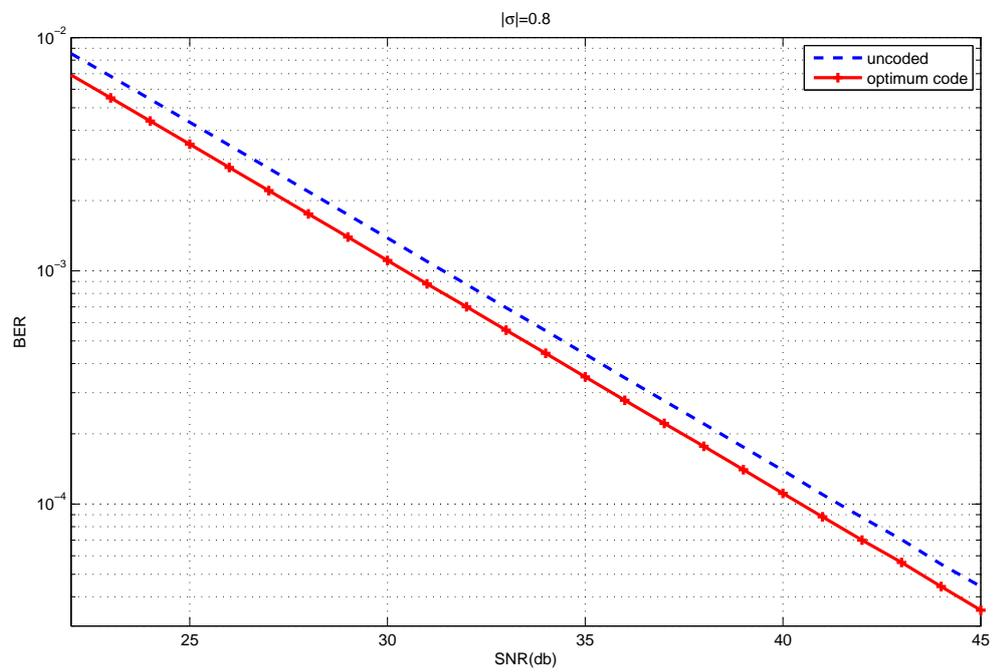
Figure 7.5: Comparison of SNR-BER when  $\sigma = 0.8e^{0.5j}$
